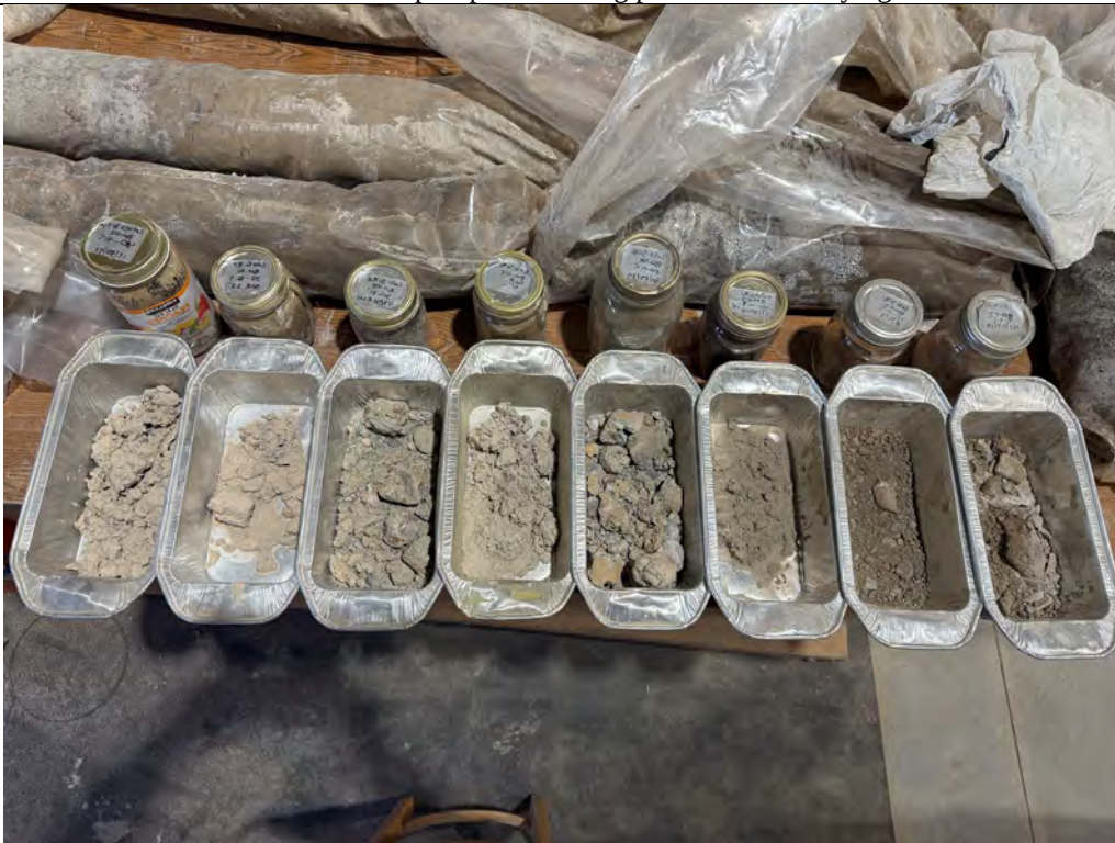
Description: BH-02 Moisture content SPT samples after being taken out the drying oven.
