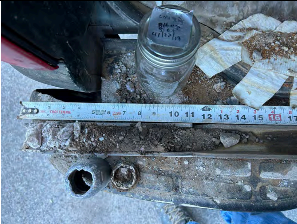
Description: BH-02 SS sample from the 5- to 6.5-foot depth.
