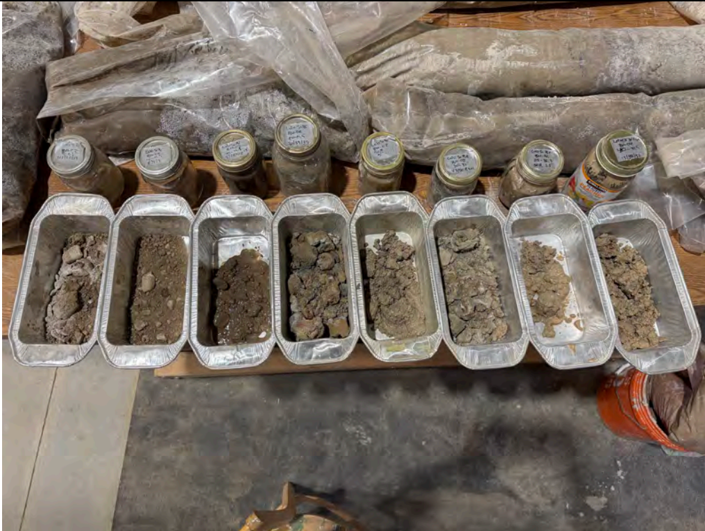
Description: BH-02 Moisture content SPT samples prior to being placed into the drying oven.
