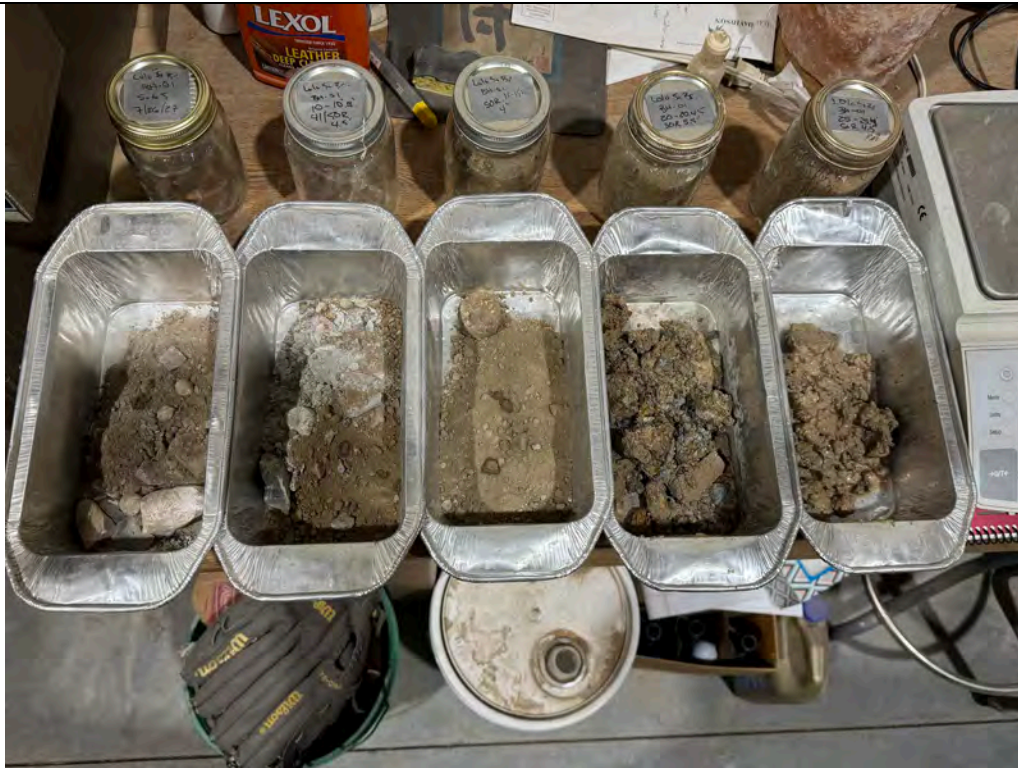
Description: BH-01 Moisture content SPT samples prior to being placed into the drying oven.
