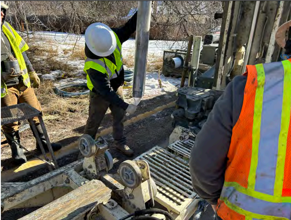
Description: BH-01 Retrieving sonic drill sample from 0 to 5 feet.
