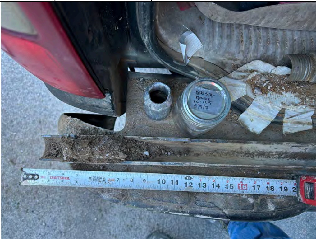
Description: BH-02 SS sample from the 10- to 11.5-foot depth.
