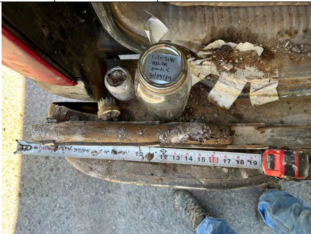
Description: BH-02 SS sample from the 20- to 21.5-foot depth.
