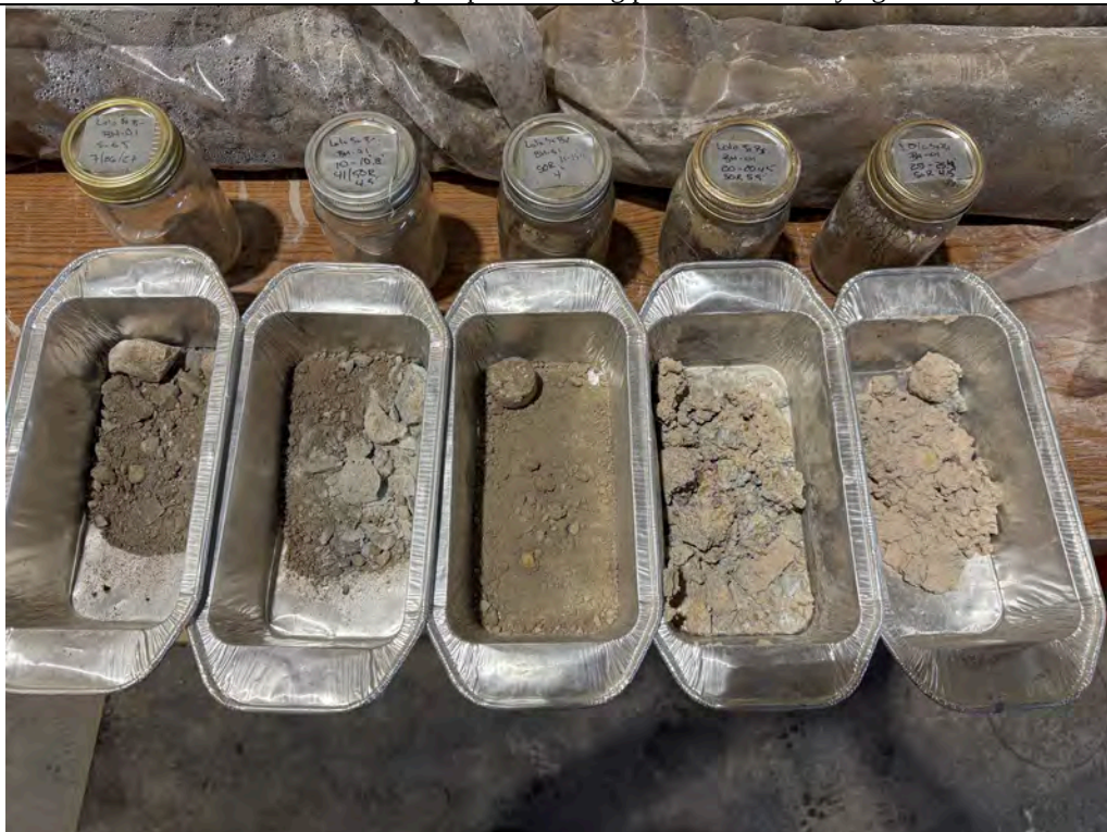
Description: BH-01 Moisture content SPT samples after being taken out of the drying oven.
