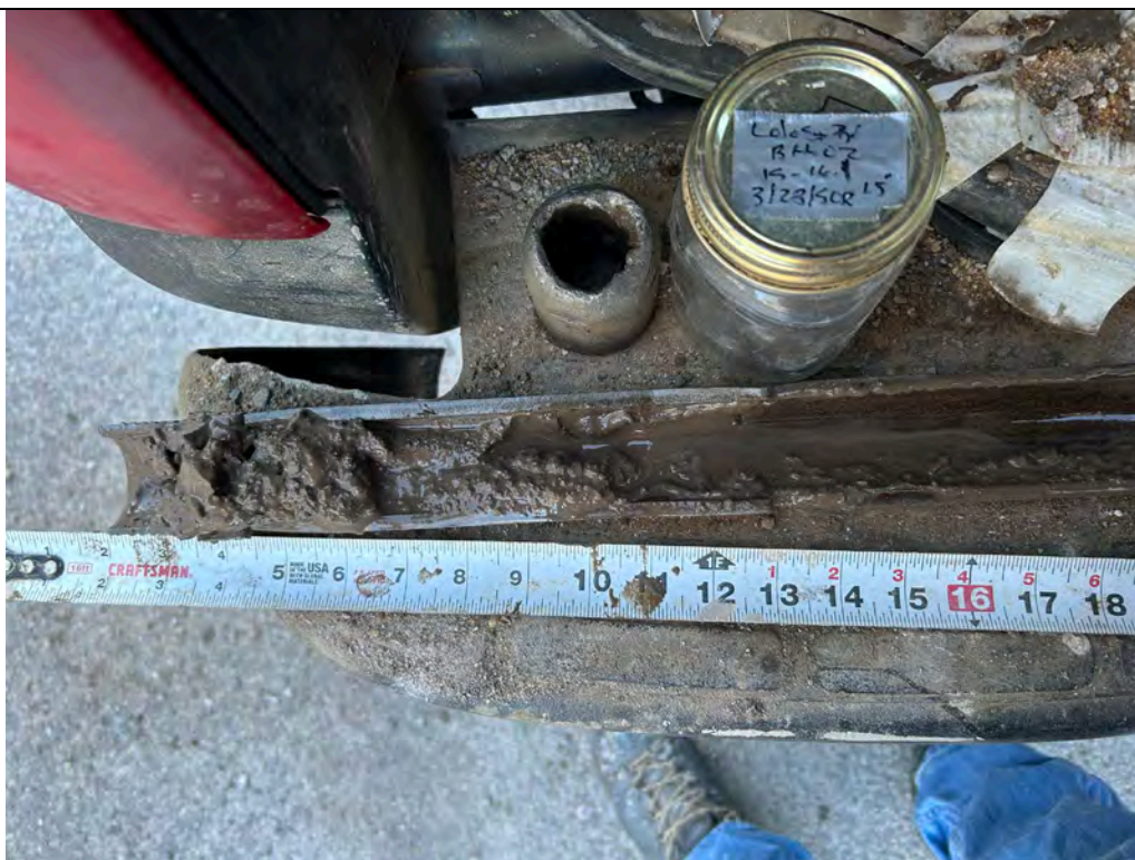
Description: BH-02 SS sample from the 15- to 16.1-foot depth.
